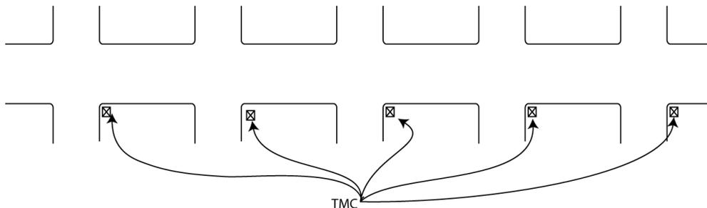
In recent years, TMC-controlled controllers have become more popular. In these systems, each controller reports back to the office, which is running traffic management software. This software can adjust timing plans based on detections, but it does not do the adjustment in real-time (as it is happening). That is, it will adjust timings for future cycles but not for the current cycle. InISync is revolutionary in its adjustment of the current cycle/demand.
