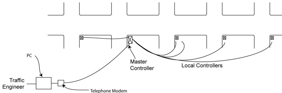
In a closed loop system, all the controllers are connected to each other using fiber optic cable. The Master Controller is connected back to the office. There are also sampling detectors on both ends and in the middle of the closed loop system. These are in addition to the inductive loop detectors used for the local controller. Multi-mode wire is run between intersections. Multi-mode wire is great for short runs.
